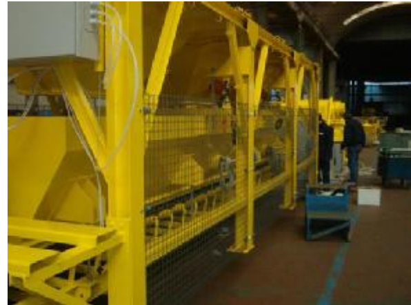
Weighting belt for raw material and conveyor belt
