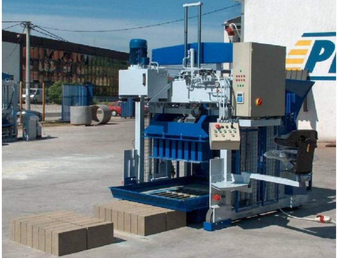
EGGLAYER 12 in process of testing of production of hollow blocks.
