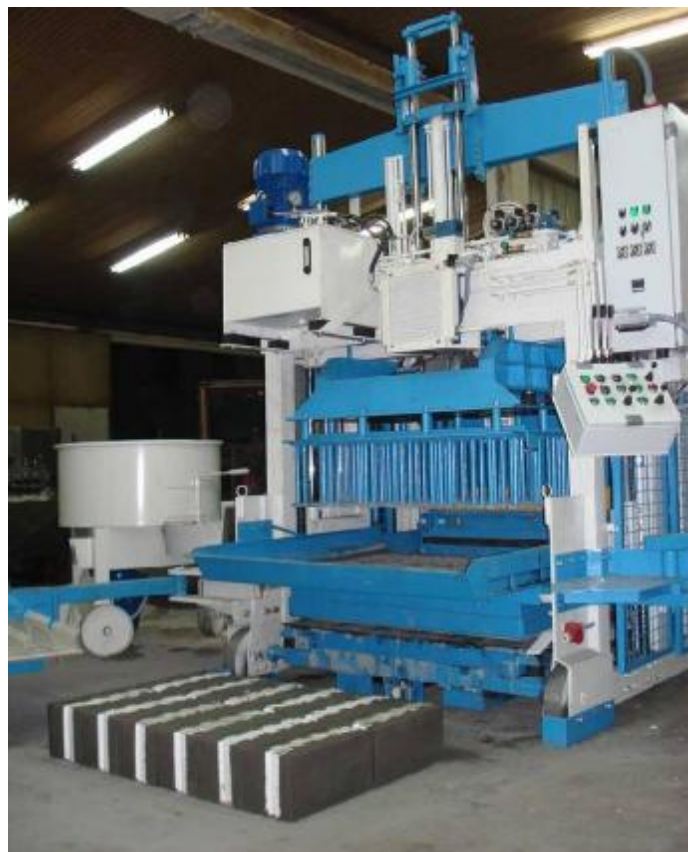
Egg layer machine EGGLAYER 12 in production of Blocks/EPS Inserts.
