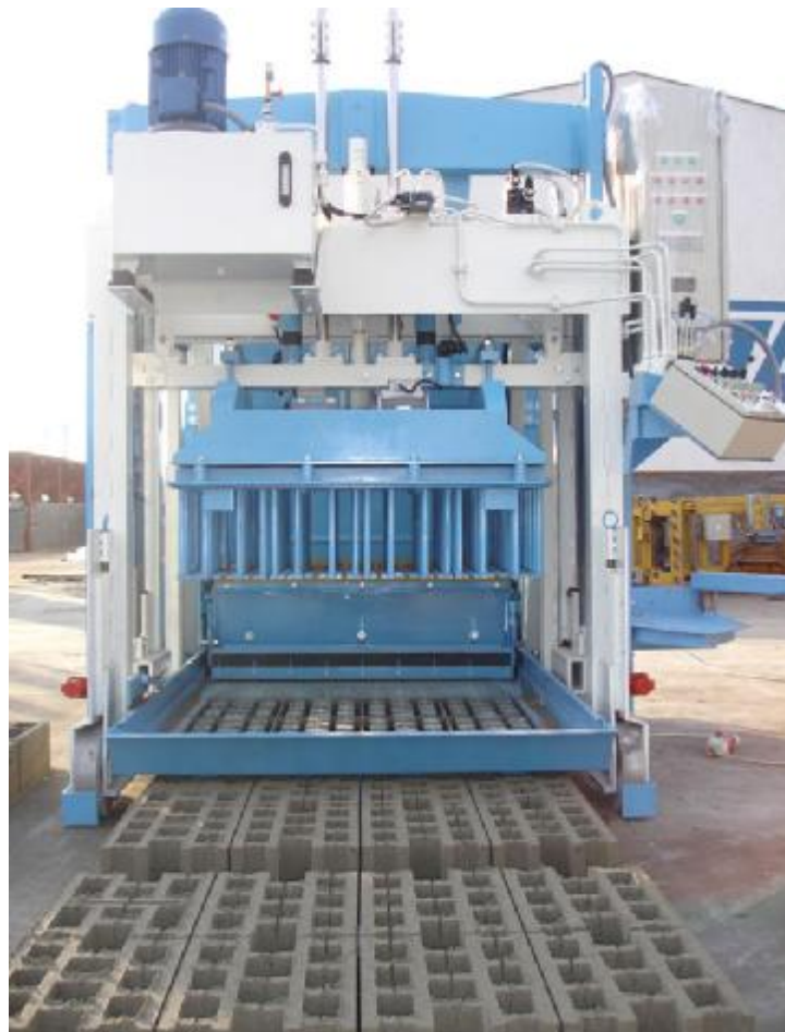
EGGLAYER 12 in process of testing of production of hollow blocks.
