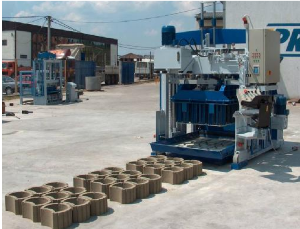
Egg layer machine EGGLAYER 12 in production of Blocks/EPS Inserts.
