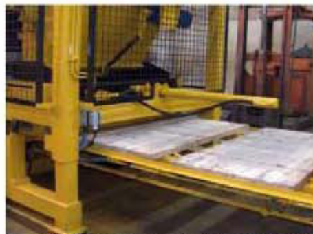
ENTER transport track with empty pallets.
