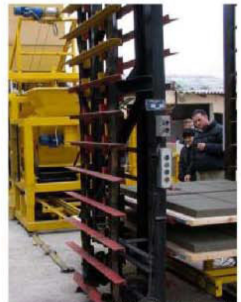
Elevator takes pallets with fresh elements.
