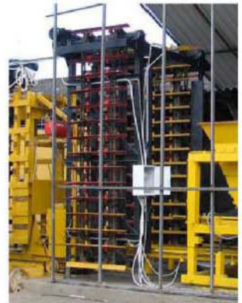
Elevator at the exit of main machine.
